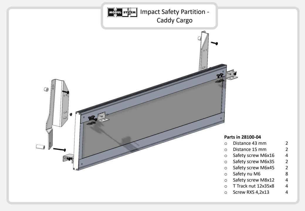
MODUL-SYSTEM Impact Safety Partition -Caddy Cargo Assembly in first and 00 second hole in the Bbeam on both sides. (23) 0 After assembly the M6 fixation apply glue on this surface to fix wall Use the fixation for the lashing eyelet for the lower bracket on both sides
